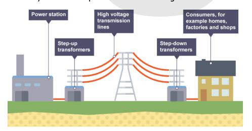
Step-up transformers increase voltage and decrease current - reducing energy losses in transmission lines making distribution more efficient.
